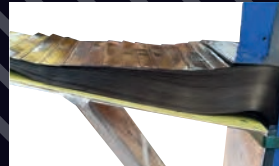
Amorphous core sheets at 25 microns thickness.
