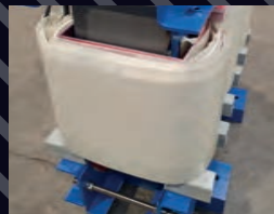
Complete core build.
