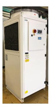
// The cooling unit ensures efficient cooling of the laser source, the optical elements and the cutting head.
