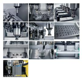
» Rapid feed speeds up to 75 m/min » Chip-to-chip time approx. 1.7 s
